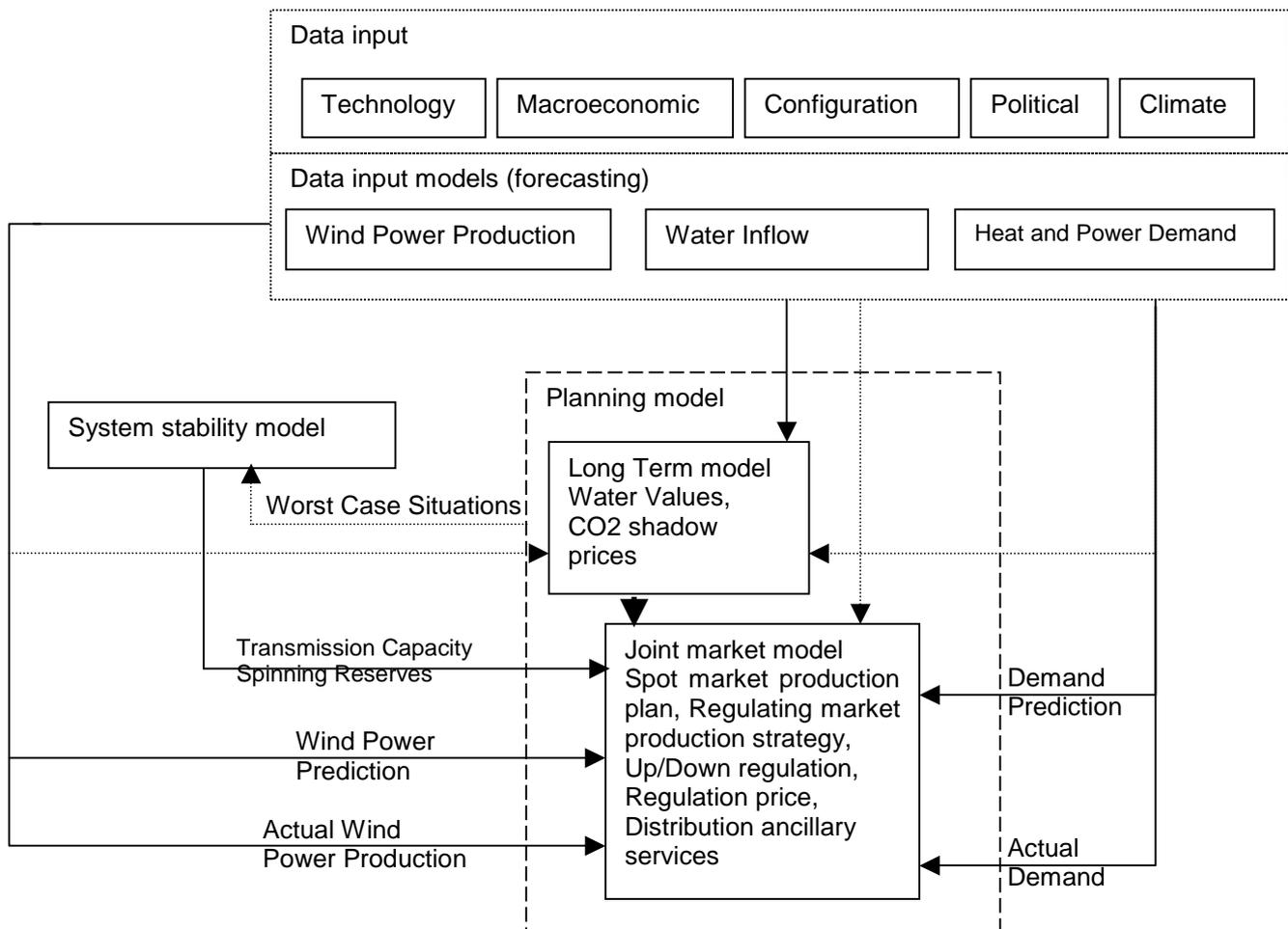
**Figure 2:** Overview of the data input and models that either provide input to the Planning model or constitute the Planning model. The models shown will exchange data and some of the data flows are illustrated in the figure.
