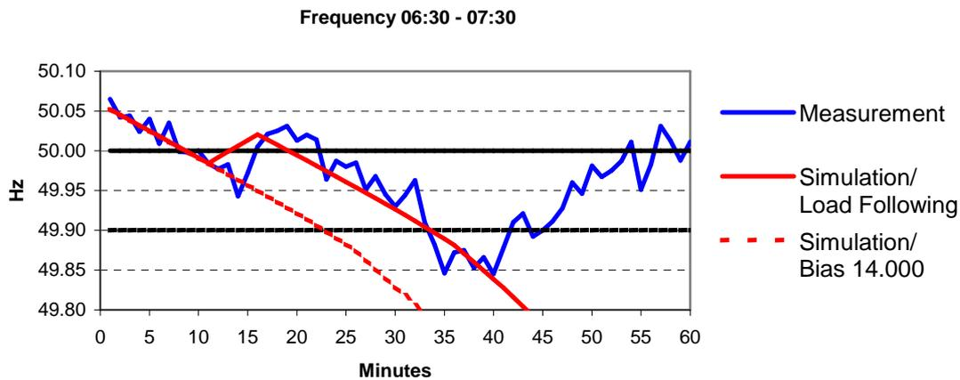
Figure 2: Measured system frequency in the Nordic system 6:30-7:30, 13 October 2003
