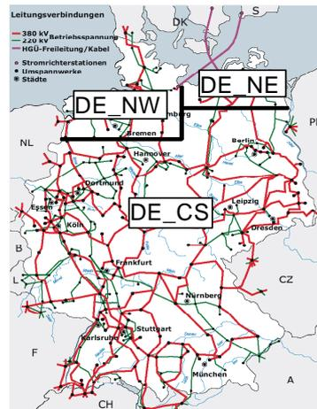
Figure 4: Subdivision of the German electricity system (VDN 2004) into three model regions.
