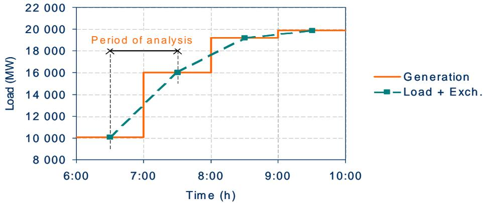
Figure 1: Period of analysis for Stepwise Power Flow simulation
