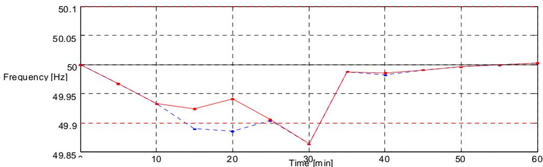
Figure 3: Simulated frequency as a consequence of less than scheduled wind power production. As all the Balancing power is used, the frequency drops below the critical 49.9 Hz limit.
