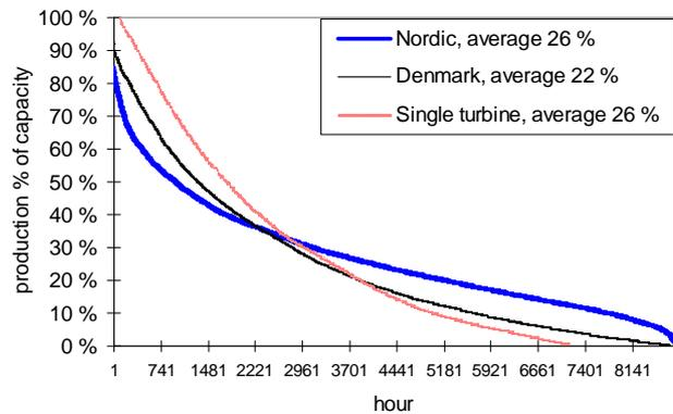
Figure 3. The effect of geographical spreading is to flatten the duration curve of wind power production. Wind energy distributed to all 4 Nordic countries is compared with one of the wind farms and one of the countries (Denmark). Average production for the curves is denoted in the legend text (year 2000 data).
