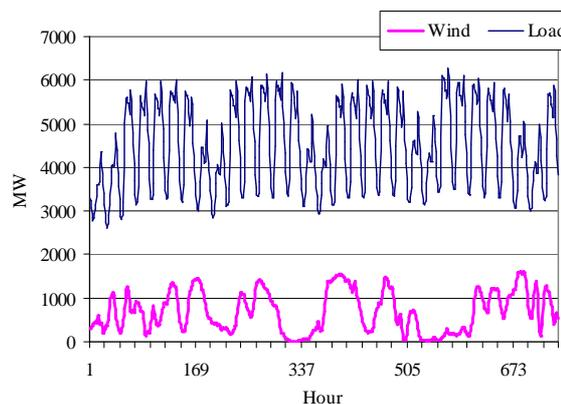
Figure 5. Electricity consumption (load) and wind power production in January 2000, for Denmark (West and East combined, 12% wind power).
