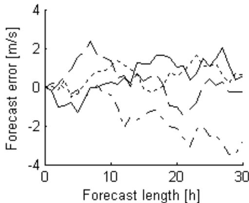
Figure 7. Four examples of ARMA (1,1)-outcomes of wind speed forecast errors.
